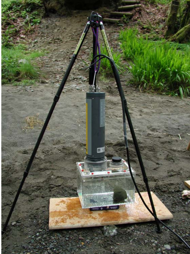
Figure 4. Clear respiration chamber with YSI Sonde used to measure gross primary production of benthic periphyton. Magnetic stirrer motor is positioned beneath chamber.
