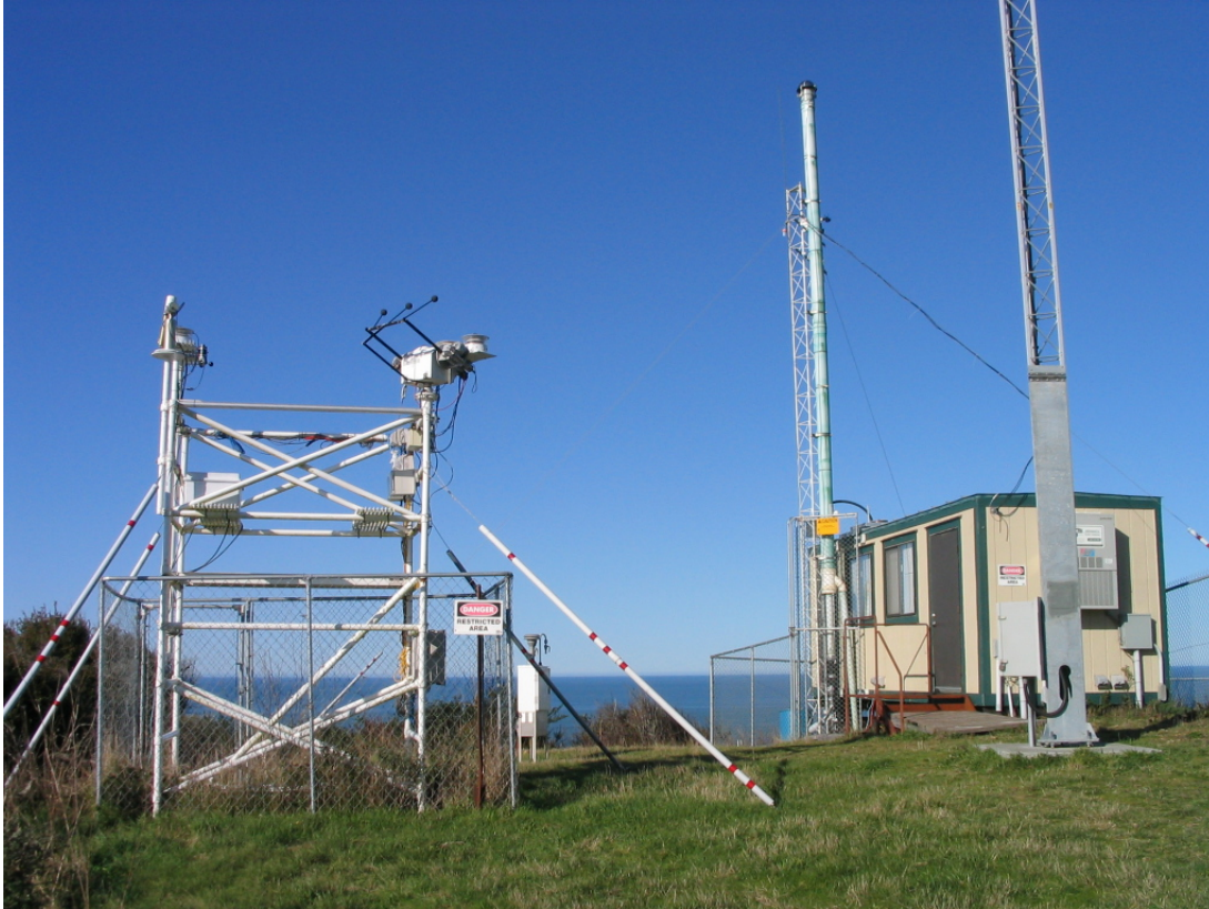
Figure 1.5. Trinidad Head Atmospheric Observatory: Latitude 40.8°N; Longitude 124.16°W; elevation 107 m. Instrumentation is housed in a 7-m long modular unit and a 10-m tower located on the top of a hill north of Humboldt Bay, Humboldt County, California.
