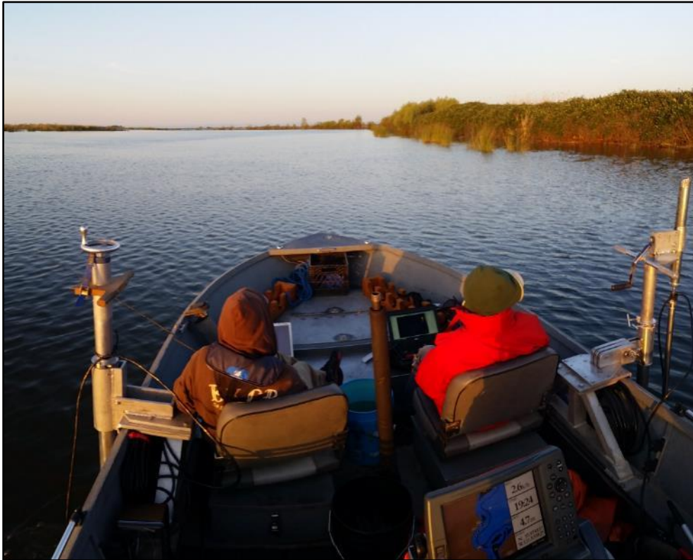
Hydro-acoustic surveys being performed using two Dual-Identification Sonar (DIDSON) cameras on the small boat “Osprey” (B. Lehman).
