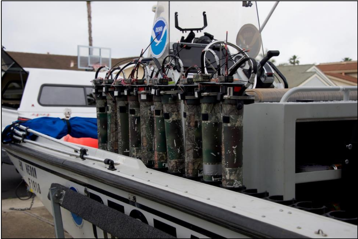
PERs mounted and ready for deployment in the small boat “Heron” (E. Danner).
