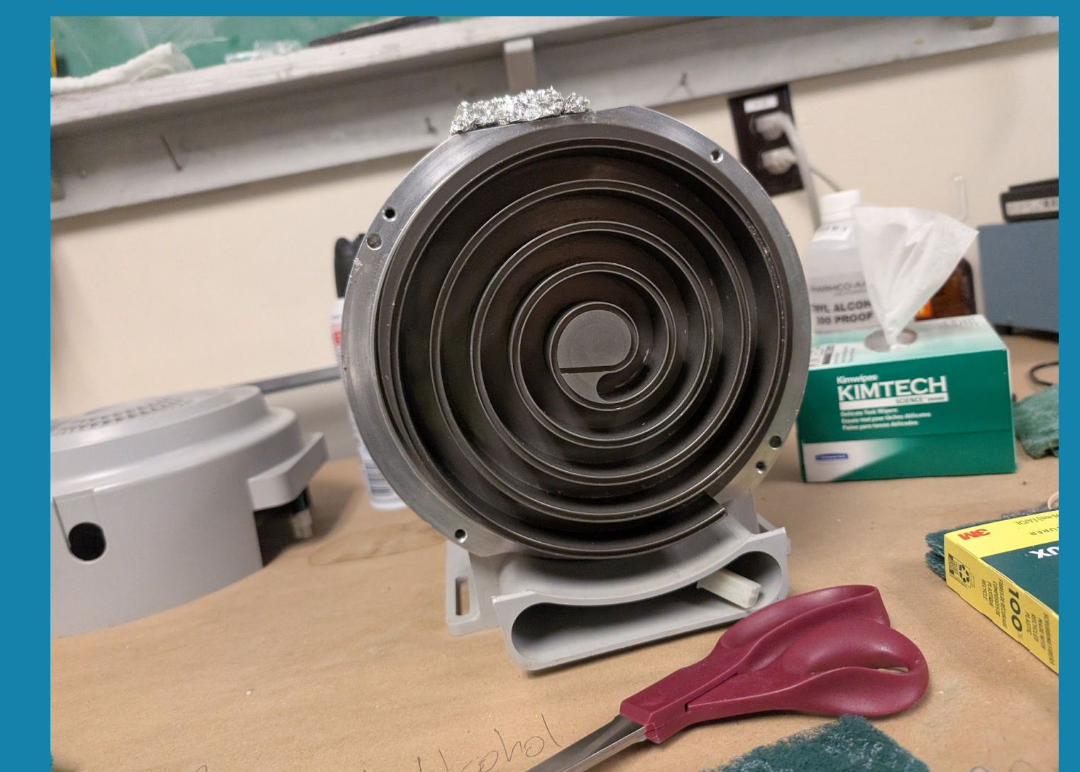
Figure 6: A photograph of a partially-disassembled roughing pump sans tip seal.
